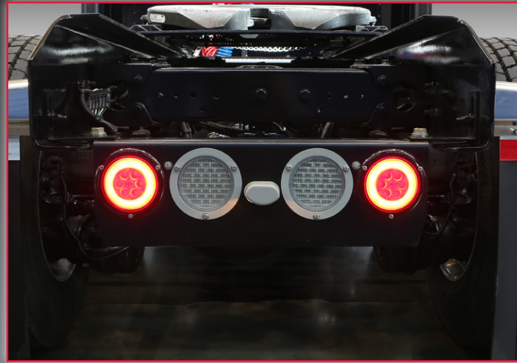
4-inch sealed LED taillights present an attractive red glow around the edges, turning bright red in the center when brakes are applied.
